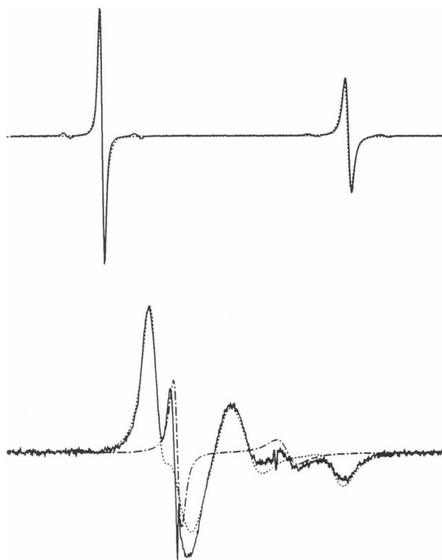
FIGURE 3 Linear EPR spectra of 5-SLE and 5-SLE bound to BSA. The top spectrum was recorded on a sample of 20 \mu M 5-SLE in 5 mM sodium acetate pH 5.0 at 20°C (EPR parameters: 40 G scan width, 0.1 G modulation amplitude (peak-to-peak), 1 mW microwave power, 1024 data points). Superimposed ( dotted line ) is a simulated spectrum with a \tau_r of 150 ps. The bottom spectrum was recorded on a sample of 20 \mu M 5-SLE/20 \mu M BSA in 5 mM sodium acetate pH 5.0 at 20°C (100 G scan width, 0.5 G modulation amplitude (peak-to-peak), other parameters same as above). Superimposed are two simulated spectra having \tau_r values of 3 ns ( dot-dashed line ) and 30 ns ( dotted line ).
